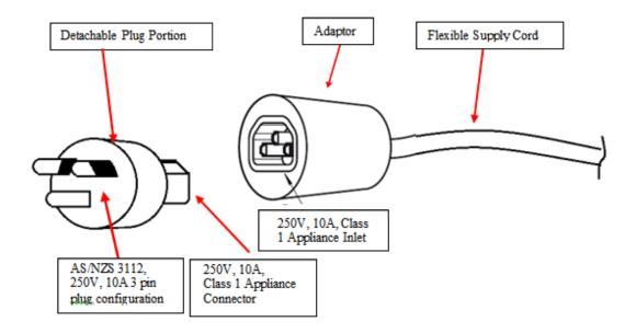
Note: the adaptor part fits within scope of AS/NZS 60320.2.2 as a plug connector
