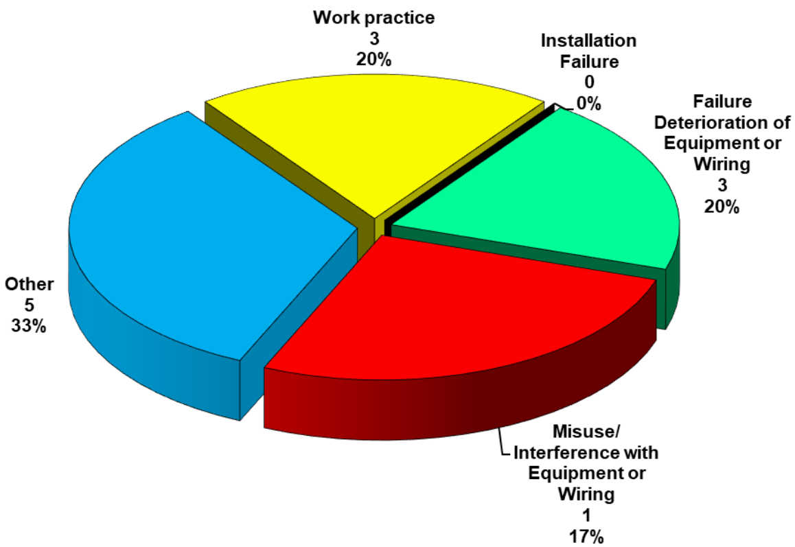
GRAPH 3.5 Deaths involving consumer installations (fixed wiring) or equipment -2020-21
